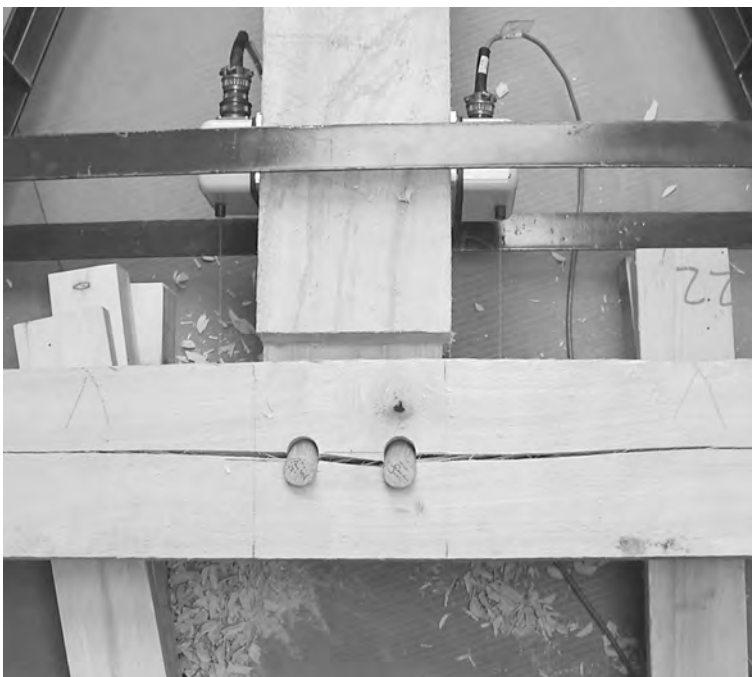
Fig. 10. Sudden failure of a mortise face during testing of a yellow poplar joint with 1-in. red oak pegs at the University of Wyoming. Timbers were 6 x 6, mortise edge distance was three peg diameters.
