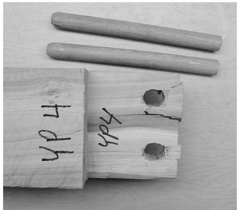
Fig. 8. Tenon relish shear failure, a brittle failure mode in pegged tension joints. Specimen did not enjoy recommended end distance and also sustained partial tensile failure, perhaps due to a material flaw.
