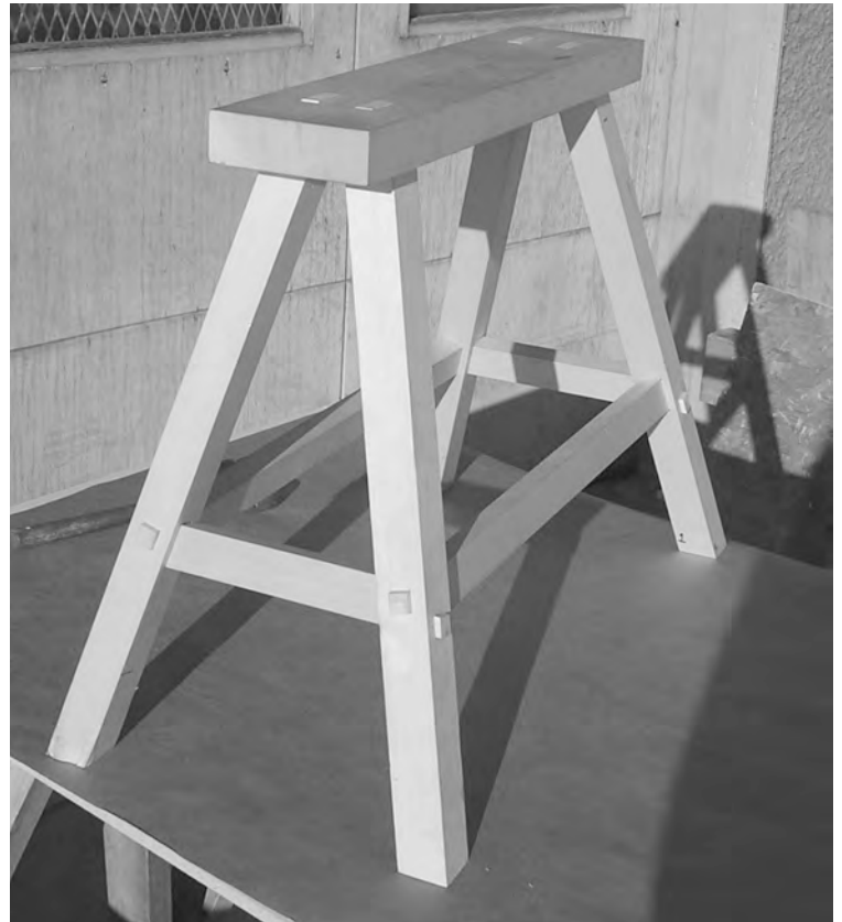
Fig. 7. Completed sawhorse with through-tenoned legs and stretchers.
